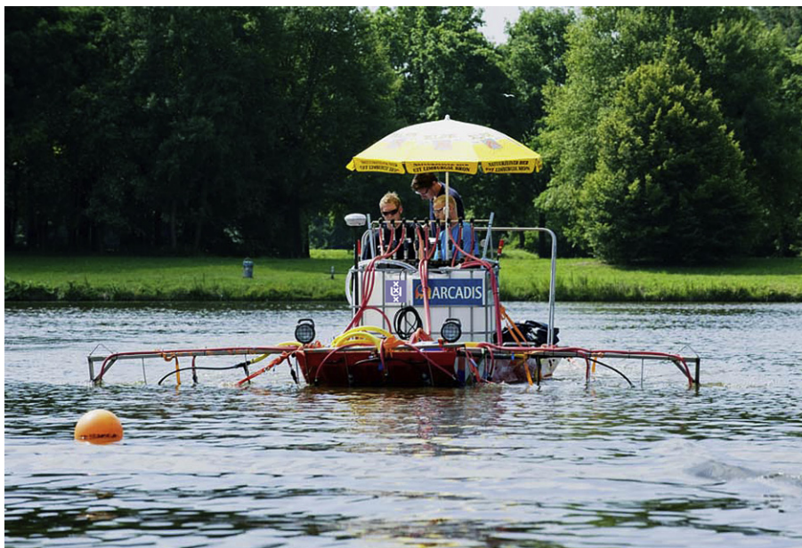
Fig. 2 – The ‘water harrow’, the device that was used to bring hydrogen peroxide into Lake Koetshuis.
